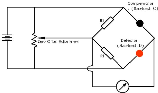
Note: The value  $R1$  is arbitrary, since the function of  $R1$  is to balance the bridge.  $1\text{ k}\Omega$  is suggested.
