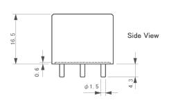
All dimensions are in mm with a tolerance of +/- 0.1 mm unless stated otherwise
