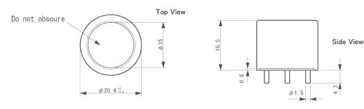
All dimensions are in mm with a tolerance of +/- 0.1 mm unless stated otherwise
