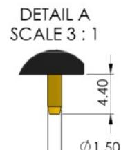
All dimensions are in mm with a tolerance of +/- 0.15 mm unless stated otherwise
