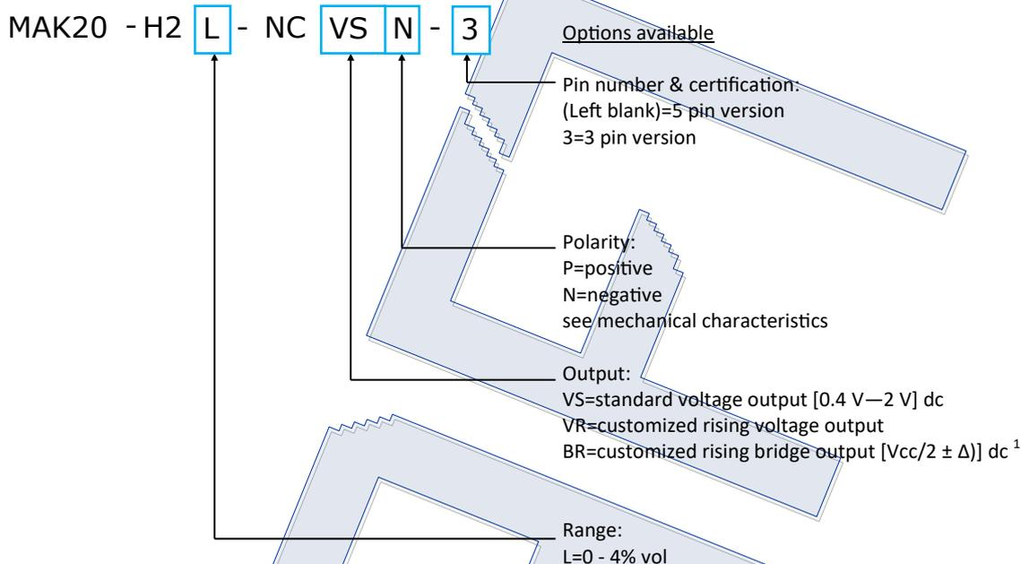
Note 1: The bridge output is indicated to use when substituting a pellistor.
